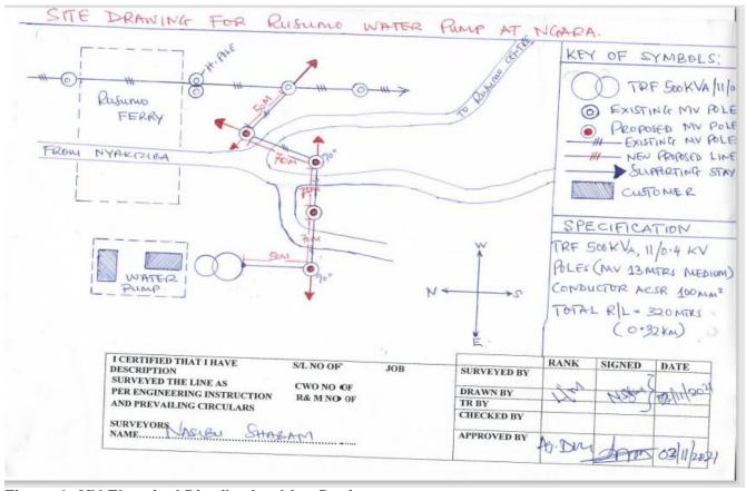
Figure 6: MV Electrical Distribution Line Design
